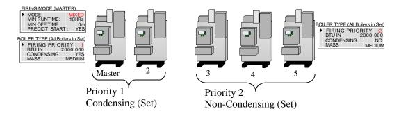
A boiler's firing priority can be designated as such in: "ADVANCED SETUP:SYSTEM:BOILER TYPE:FIRING PRIORITY: 1" menu on each boiler. A priority of '1' is the highest priority, a '2' the lowest (default is always 2).
